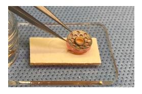
• The back plate is placed on the stem of the front plate.
