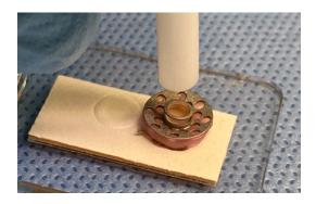
• The hollow end of the assembly tool is used to press the locking ring firmly down into the groove, usually with an audible snap. The assembly tool must be at 90 degrees from the front plate when pressing down.
