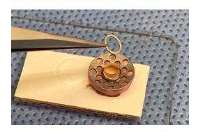
The locking ring is placed on stem of the front plate and properly aligned parallel to the front plate prior to final assembly.
